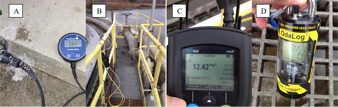
Figure 2: (A) D.O. level at Speece Cone discharge, (B) Sensors over primary weir, (C) D.O. reading at primary weir, (D) H<sub>2</sub>S reading at primary weir
